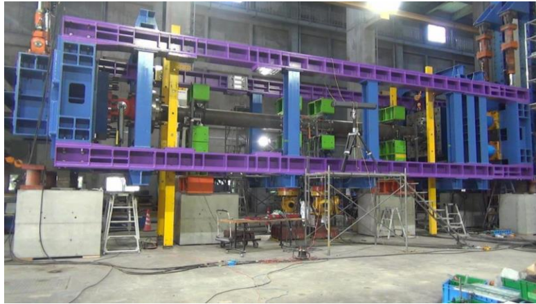
Fig. 1 Bending test of hollow CFST pile
